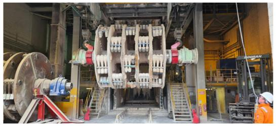
With a total weight of 80T, rotor lifting was courtesy of a pair of tandem-controlled 41T SWL wire rope hoists located on monorail beams arranged at 90° to the rotor bearing journal stub shafts.
