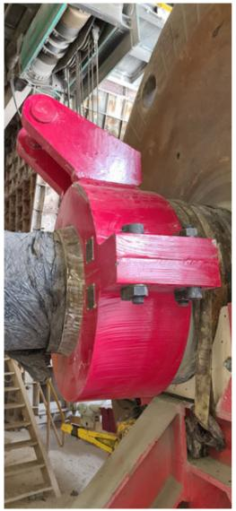
Hoist & Winch designed and manufactured two 41T SWL rotor lifting lugs to assist the lifting process.
