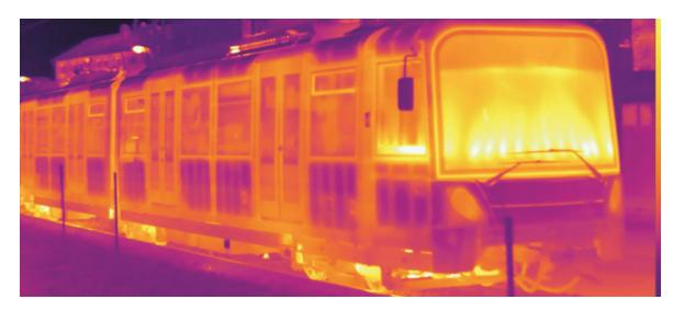
With the help of **thermal imaging**, it is possible to quickly and safely locate any heat sources caused by errors. This is mainly applied to the following components
