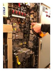
act, which jam in front of the moving train. The pressuretightness of the cabin protects the train passengers from serious injuries. The ii900 makes it very easy to control the pressure tightness. By "lighting" the possible leaks, such as entrances, windows, air conditioning or bulkheads.
